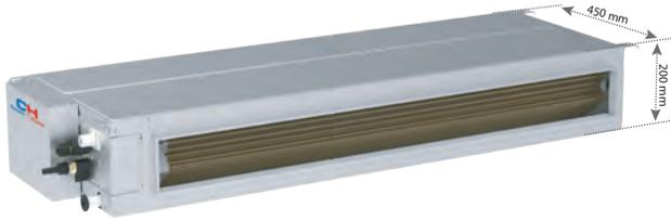
High static pressure duct units ranging from 7.1 kW to 8.5kW are only 900mm in length. They are suitable to be installed in corridors whose width is  $\leq 1.2\text{m}$ .
