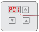
Water inlet temp. Sensor failure
