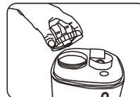
2. Turn the water tank upside down and unscrew the tank cap.
