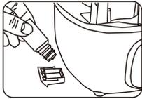
4. If you would like to use the aroma diffuser function, drop some essential oil in the aroma diffuser tray. **DO NOT** put the essential oil directly into water tank.
